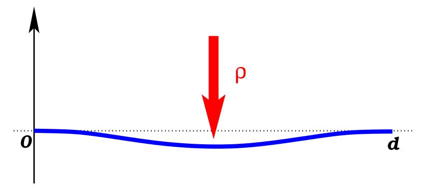
Two end-points are fixed, and clamped so that they are level, e.g.
