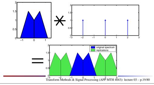
Even though the input signal is band limited, the resulting spectra overlap, because the maximum frequency  $f_c > 1 = f_s/2$ . The overlapping is a problem which we must avoid.
