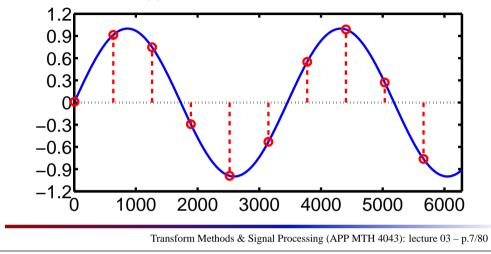
The x-axis is discretised, but the y values are still exact. We have sampled the function at a set of sample points.
