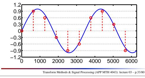
Some background: all **digital** data is represented as numbers, e.g. the data on a CD is represented as numbers. The numbers are usually represented in some binary format, for instance, we might write a number in terms of binary "bits" where each bit is either 0 or 1
