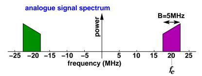
To include entire spectrum, we need to sample at  $2 \times 22.5 = 45$  MHz.
