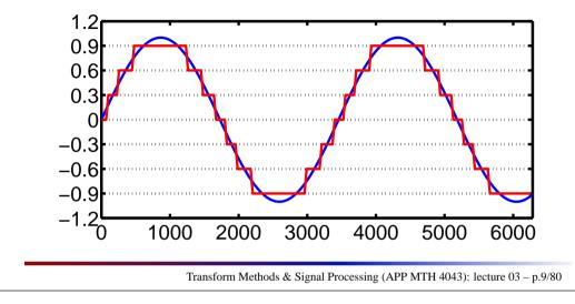
Given a set of sample points, we can try to reconstruct the original continuous signal in a number of ways (this is called interpolation). The illustration is a simple (but crude) method where we assume the signal takes the value of the sample until we get to the next sample. This is sometimes called nearest neighbor, or piecewise constant interpolation.
