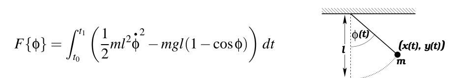
The kinetic energy is in the appropriate form, and the potential does not depend on time, so the pendulum system conserves energy, e.g.
