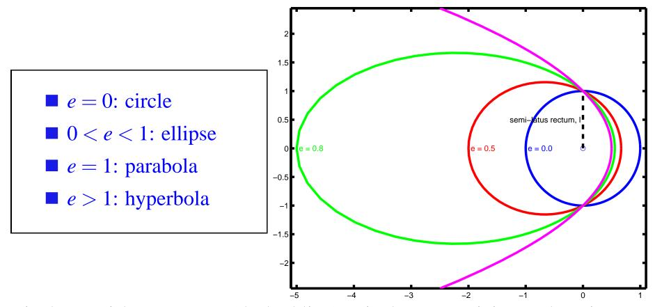
*L* is the semi-latus rectum (dashed line), *e* is the eccentricity, and  $\omega$  gives the angle of the perihelion (point of closest approach) which is zero in the above figure.
