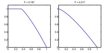
The shape doesn't satisfy a common requirement for such nose cones that they be tangent to the base cylinder where they touch, but we haven't really considered that constraint yet (and Newton's solution doesn't meet this criteria either).
