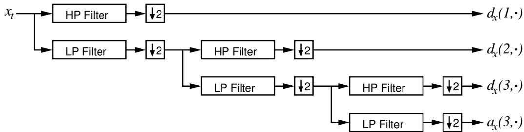
Fig. 2. The filter-bank. At each level in the recursive structure, the High Pass (HP) output:  $d_x(j, \cdot)$ , and the Low Pass (LP) output:  $a_x(j, \cdot)$ , occur at half the rate of the input  $a_x(j-1, \cdot)$ .
