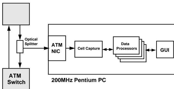
Fig. 3. The architecture of the ATM monitor.
