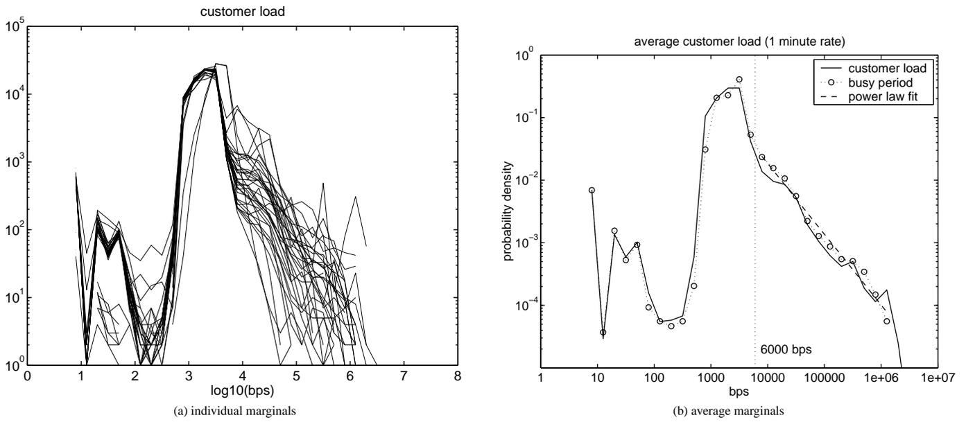
Fig. 8. Plots of the marginal distributions of the individual cable modems sampled from data set (a). Note the log-log axis.
