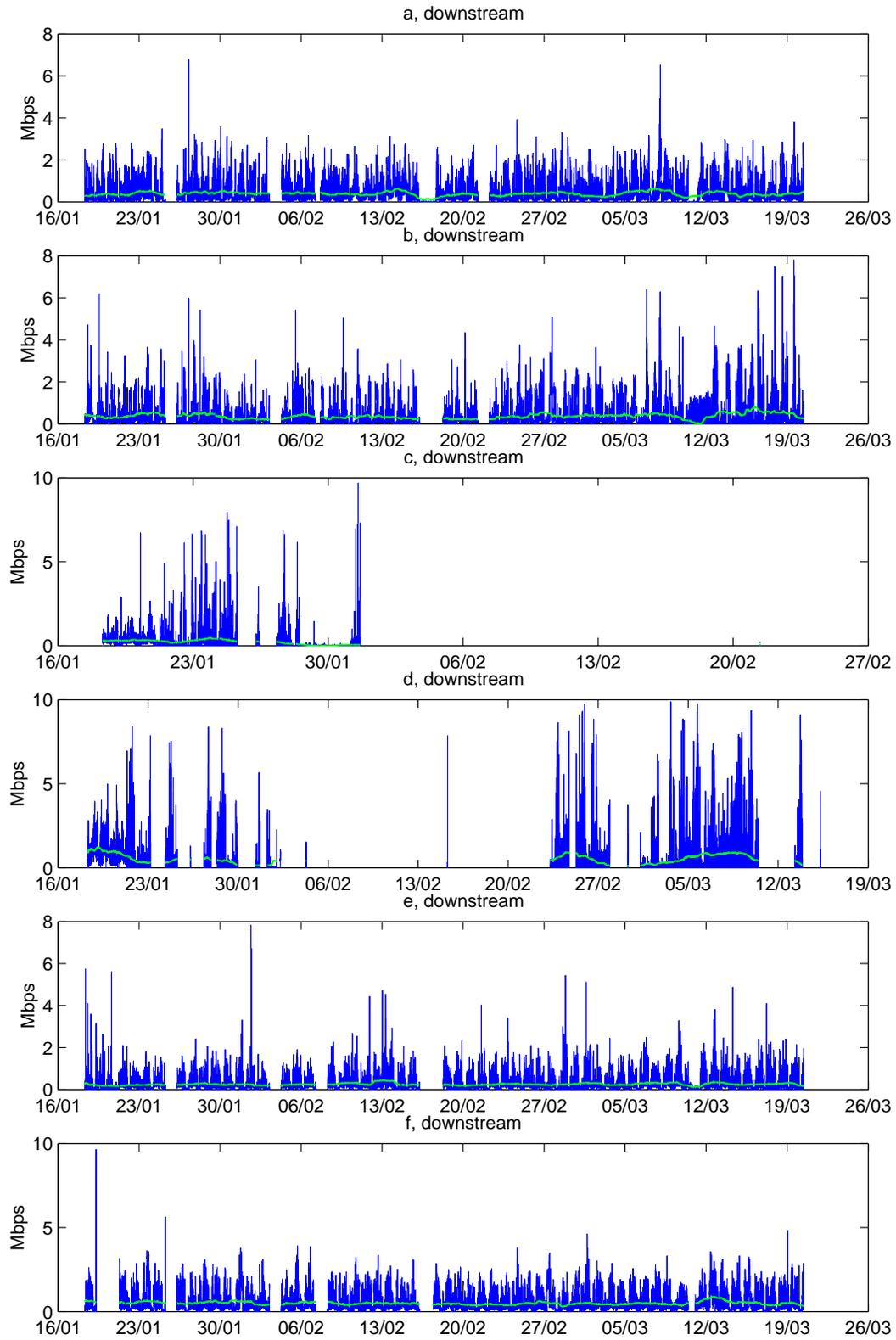
Fig. 2. Downstream CMTS traffic. The solid line shows one minute average rates (in Mbps) and the pale line shows a two week moving average of the data rate.
